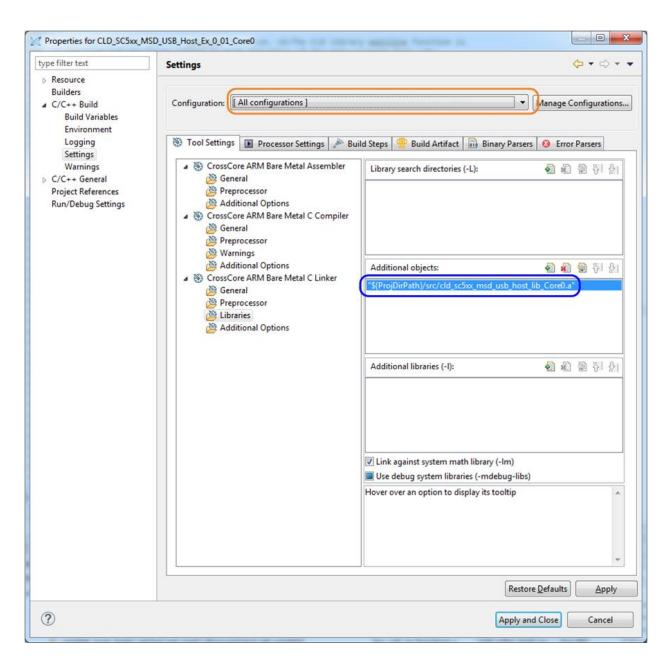
5. The 'Additional objects' setting needs to be set for all configurations (Debug, Release, etc). This can be done individually for each configuration, or all at once by selecting the [All Configurations] option as shown in the previous figure (circled in orange).
